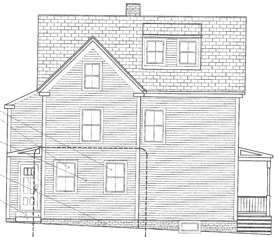
4 NEW SIDE ELEVATION 1/8" = 1'-0"
