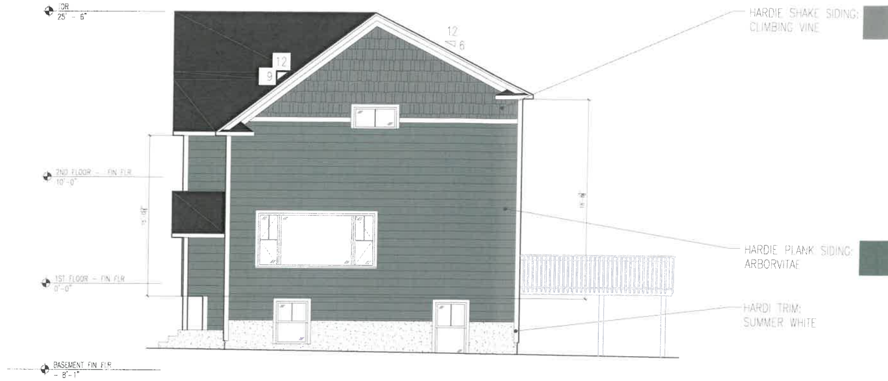
EAST EXTERIOR ELEVATION
