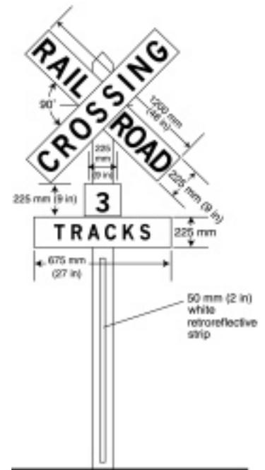
FIGURE 5.24 Highway-rail crossing (Crossbuck) sign (MUTCD Fig. 8B-1)
