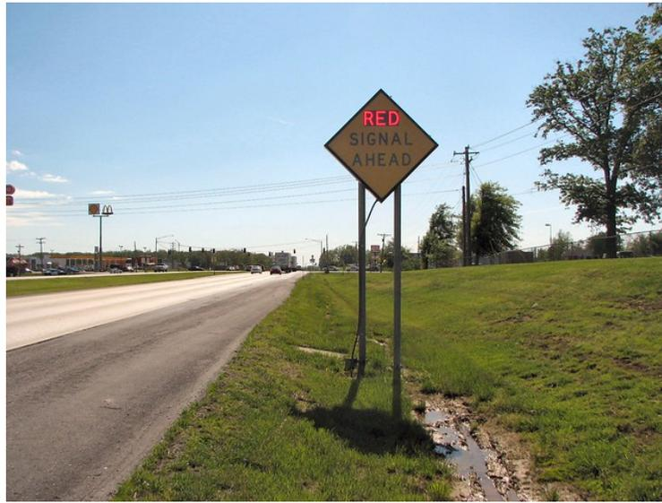
Example of Advanced “Red” Signal Ahead” activated bank-out sign Assembly
